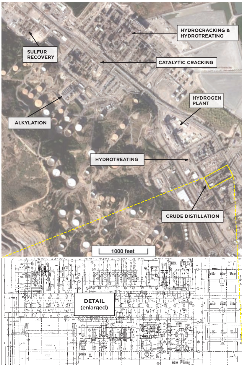
A refinery's processing equipment viewed from the sky. Chevron Richmond processing yards. Detail: Crude distillation unit schematic illustrates equipment components in a refinery process unit. Images from City of Richmond permit files and EIR SCH #2011062042.
