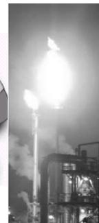
Flares were routinely abused to burn off “waste” gas in the past, despite availability of equipment to recycle gases, resulting in emissions of many tons per day.
