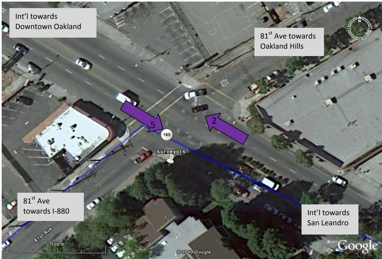
Figure 18. 81<sup>st</sup> Ave and International Blvd. Red arrow: >400 trucks; yellow arrow: 200-400 trucks; blue arrow: 100-200 trucks; purple arrow: <100 trucks. The table below shows the truck volumes for each direction of movement. Total consists of 1 weekday afternoon of counting, approximately 1pm-5pm. Blue line indicates the Oakland truck route.
