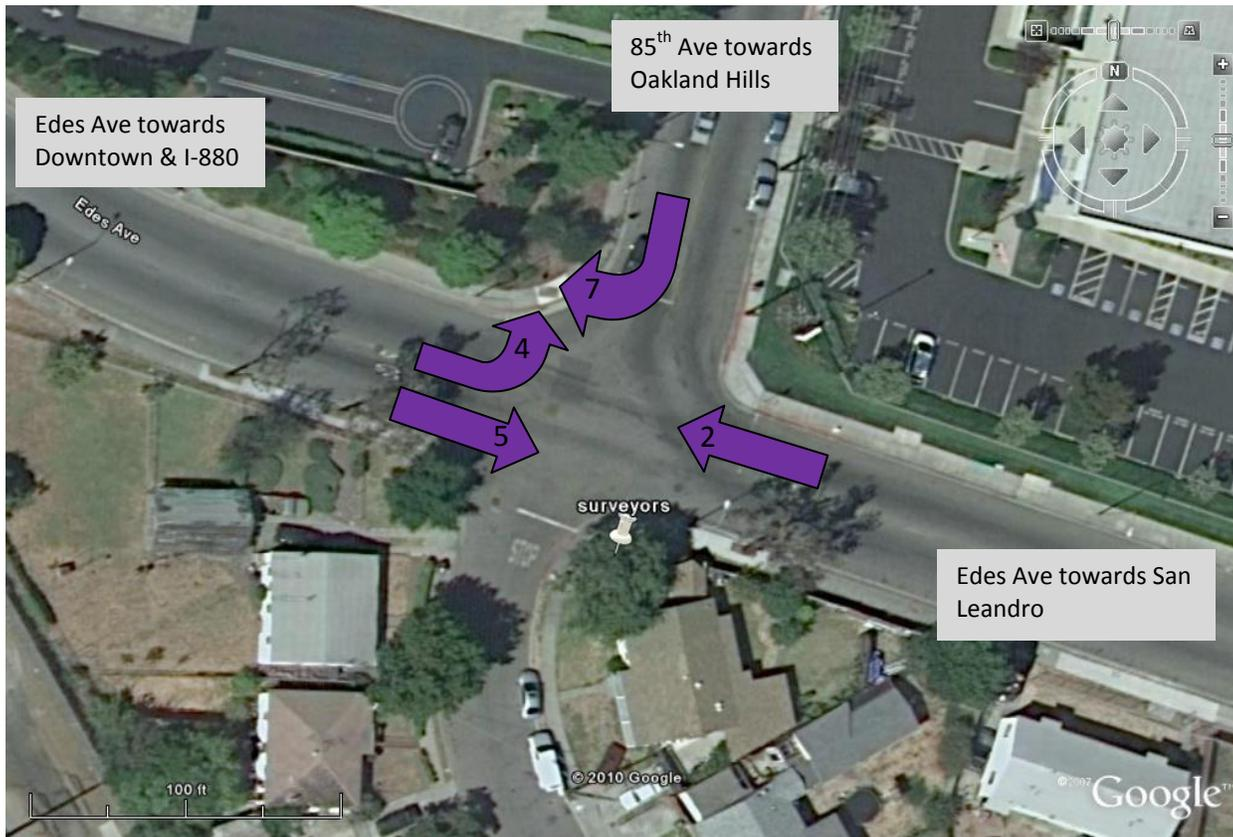
Figure 20. 85<sup>th</sup> Ave and Edes Ave. Red arrow: >400 trucks; yellow arrow: 200-400 trucks; blue arrow: 100-200 trucks; purple arrow: <100 trucks. The table below shows the truck volumes for each direction of movement. Total consists of 2 weekday afternoons of counting, approximately 1pm-5pm.
