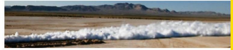
**8,300 lb. desert test showed HF forms ground-hugging lethal vapor cloud.** Exposure to the MHF plume during a major release can cause serious irreversible health effects 16-17 miles downwind from the Torrance or Valero refineries. In the first 8-9 miles death can occur. (Based on EPA's Risk Management Program guidelines.)
